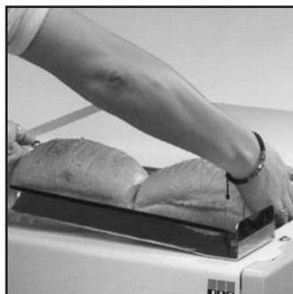
The loaves are loaded once the front-loading cover is open. As the cover locks, the loaves are sliced automatically and exit through the upper opening, right next to the bagging device.
