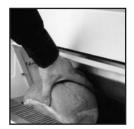
A safety bar on the loading side protects the operator when placing the loaves.
