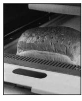
Available as an option, an automatic and retractable loaf pusher helps slice the last loaves.
