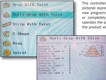
The controller features a list of stored programmes together with a pictorial representation of the product. By moving beyond this screen new programmes can be created, or existing programmes 'tweaked', or completely changed. To make programming really easy for the operator the product creation screen shows a pictorial representation of the product with dimensions in millimetres. The programmes are pass-
