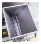
Intermediate gears are used in conjunction with the soft mix hopper, soft mix gears. Intermediate gears are placed into the hopper above the standard soft mix gears to help drive mix of intermediate consistency through the nozzles.
